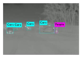
The example of traffic obstacles detection algorithm operation based on LWIR stereo camera data processing
