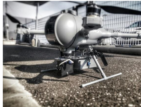
Drone mounted gamma rays and nerve gas sensors
